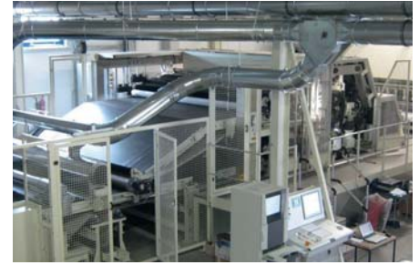
This line produces hygiene nonwovens for diapers.
