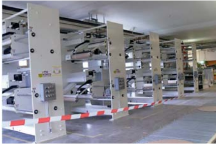
Unwinder, cutter, spool stand, winder: This line cuts basic rolls into strips. Used by hygiene product manufacturers.
